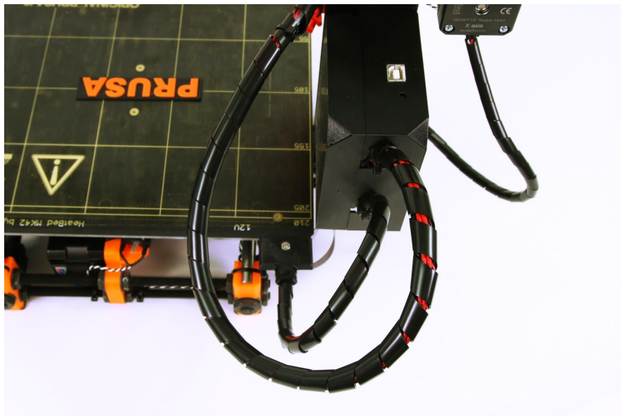
Pict. 46 - Cables should be wrapped in a spiral wrap
