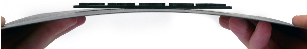
Pict. 14 - Removing the model from the PEI print surface by bending the steel sheet.
