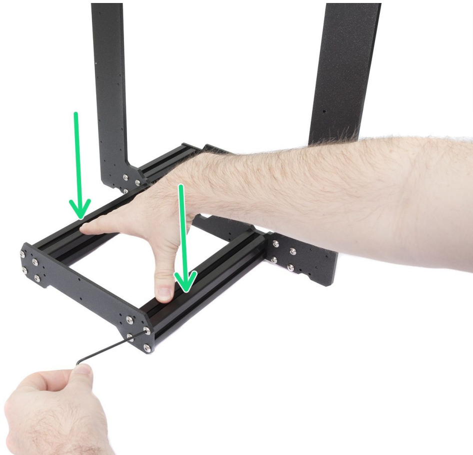
Pict. 42 - Proper way to tighten the frame, plates and aluminium extrusion together.
