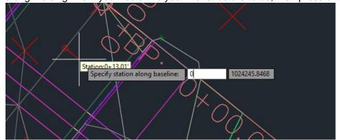
Once you've chosen how far along the allignment to place the structure, you'll have to type in the offset. This determines how far from the center point the structure will be placed. Then press enter.
