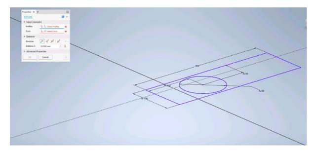
This will essentially extend your 2D sketch into a prism. This has similar options to the dimension tool as far as how far to extrude the object..
