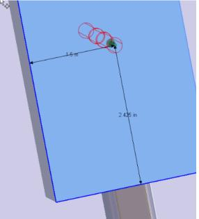
select two edges to reference the distances for the bolt.
