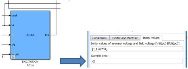
Some model blocks will open a sub-model when double-clicked – to expose the inner workings of the block.
