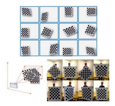
The Calibrator works with a range of checkerboard square sizes. As a general rule, your checkerboard should fill at least 20% of the captured image. For example, the preceding images were taken with a checkerboard square size of 108 mm.
