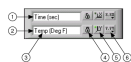
Figure 5.13: 1. X-axis, 2. Y-axis, 3. Scale Labels, 4. Scale Lock Button, 5. Autoscale Button, 6. Scale Format Button
