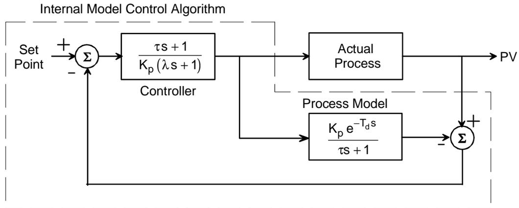
Since the basic premise of the Smith Predictor and IMC are identical, we can expect the behavior to be identical, when applied to the same process.
