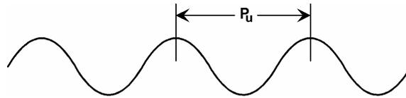
$K_{cu}$  = Controller Gain that causes sustained oscillation
