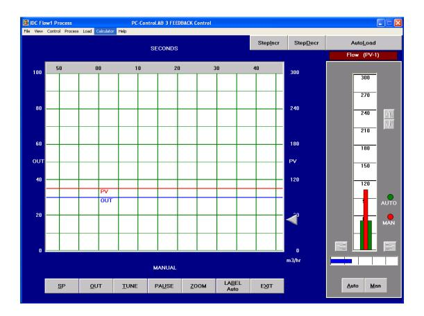
This display gives a general idea of the process and displays the major variables PV (process variable scaled 0 to 300 m3/hr) and OP (controller output signal to flow control valve scaled in range 0 to 100%). The SP (set point) is shown as an arrow on the right of the trend screen and as a red bar on the controller faceplate.
