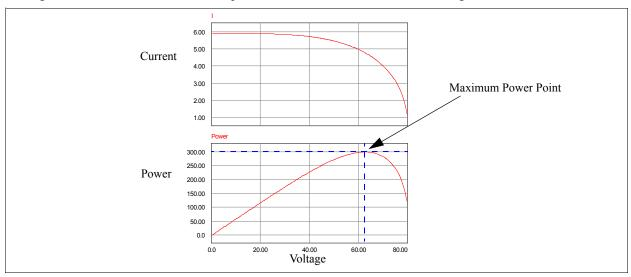
As shown in the figure, as the voltage increases, the solar module output power increases. At one point, the output power will reach the maximum. Many control schemes have been proposed to track the maximum power point (so called Maximum Power Point Tracking, or MPPT) under different operating conditions. Several MPPT examples have been included in the PSIM example set.
