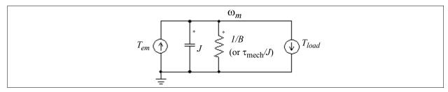
This circuit shows that the mechanical time constant  $\tau_{mech}$  is equal to the RC time constant of the resistor 1/B and the capacitor J. Therefore, the mechanical time constant can be measured by the following test:
