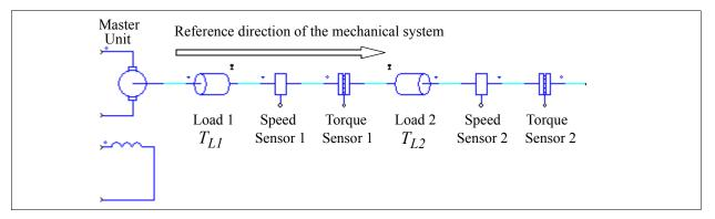
In this mechanical system, the machine on the left is the master unit. The reference direction of the mechanical system is from left to the right along the mechanical shaft. Comparing this direction with the reference direction of each element, Load 1, Speed Sensor 1, and Torque Sensor 1, will be along the reference direction, and Load 2, Speed Sensor 2, and Torque Sensor 2 will be opposite to the reference direction of the mechanical system.
