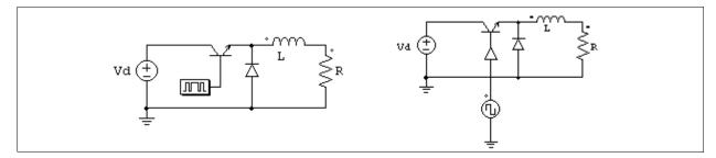
The following shows another example of controlling the BJT switch. The circuit on the left shows how a BJT switch is controlled in the real life. In this case, the gating voltage  $V_B$  is applied to the transistor base drive circuit through a transformer, and the base current determines the conduction state of the transistor.
