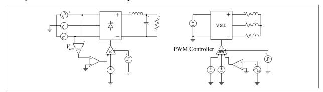
The thyristor circuit on the left uses an alpha controller. For a three-phase circuit, the zero-crossing of the
