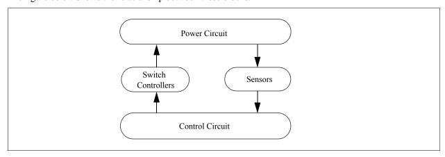
The power circuit consists of switching devices, RLC branches, transformers, and coupled inductors. The control circuit is represented in block diagram. Components in s domain and z domain, logic components (such
