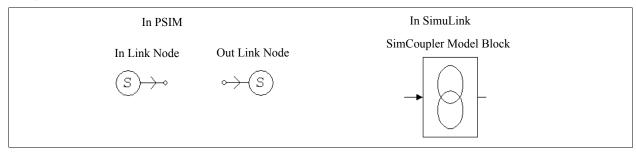
In PSIM, the In Link nodes receive values from Simulink, and the Out Link nodes send the values to Simulink. They are all control elements and can be used in the control circuit only. In Simulink, the SimCoupler model block is connected to the rest of the system through input/output ports.
