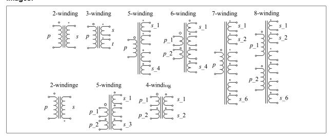
In the images, p refers to primary, s refers to secondary, and t refers to tertiary. The winding with the largest dot is the primary winding or first primary winding. For the multiple winding transformers, the sequence of the
