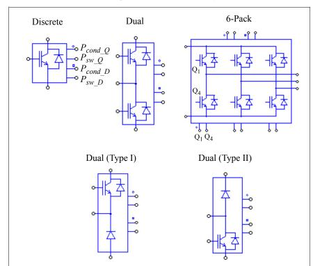
In the images, beside the IGBT and diode terminal nodes, there are four extra nodes from the top to the bottom (or from the left to the right on the top for the 6-pack package). They are the nodes for transistor conductor losses  $P_{cond\_Q}$  (the node with a circle), for transistor switching losses  $P_{sw\_Q}$ , for diode conductor losses  $P_{cond\_D}$  (the node with a square), and for diode
