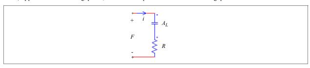
The mmf, in the form of a voltage source, applies across the capacitor (the capacitance has the value of the inductance factor  $A_L$ ) and the resistor R. For the element  $Air\ Gap$ , the inductance factor can be calculated from the air gap length and the cross section area as:
