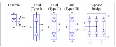
In the images, beside the diode anode and cathode terminals, there are two extra nodes. The node with a dot is for the diode conduction losses  $P_{cond}$ , and the node without a dot is for the diode switching losses  $P_{sw}$ .
