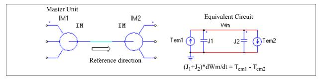
Similarly, if we define the machine IM2 as the master unit, the reference direction of the overall mechanical system will be from right to left, as shown below. Based on this direction, the machine IM1 will be opposite to the reference direction, and the machine IM2 will be along the reference direction. This leads to the equivalent circuit of the mechanical system as shown on the right.
