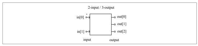
The node sequence is from the top to the bottom.
