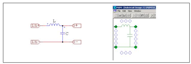
In this case, the inductance and capacitance values will be defined through the interface, and need to appear in the property window of the new LC filter element. Therefore, the parameter value for the inductance needs to be defined as a variable, in this case, L, and the value for the capacitance as C.
