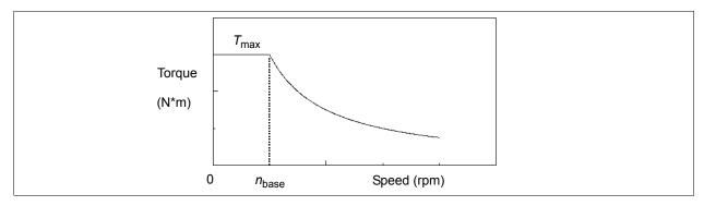
When the mechanical speed is less than the base speed  $n_{\text{base}}$ , the load torque is:
