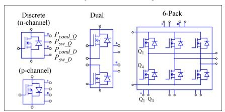
In the images, beside the MOSFET and diode terminal nodes, there are four extra nodes from the top to the bottom (or from the left to the right on the top for the 6-pack package). They are the node for transistor conductor losses  $P_{cond\_Q}$  (the node with a circle), for transistor switching losses  $P_{sw\_Q}$ , for diode conductor losses  $P_{cond\_D}$  (the node with a square), and for diode switching losses  $P_{sw\_D}$ , respectively.
