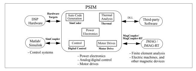
The PSIM simulation environment consists of the circuit schematic program PSIM, the simulator engine, and the waveform processing program Simview<sup>1</sup>. The simulation process is illustrated as follows.
