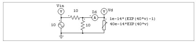
The nonlinear element (NONI) in the circuit above models a nonlinear diode. The diode current is expressed as
