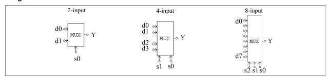
In the images, d0..d7 are the data inputs; and s0..s2 are the control signals. The truth tables of the multiplexers
