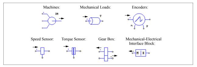
The reference direction of each element and the reference direction of the overall mechanical system determine how the element interacts with the mechanical system.
