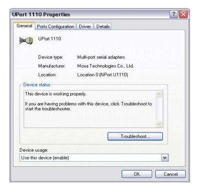
Select the 'Ports Configuration' tab and note the COM port that has been allocated to the UPort 1110.
