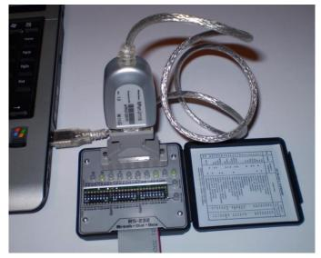
Normally in a hands-on situation you would do this by observing the LEDs on the breakout box or by measuring the voltage across the two pins (TxD on pin 2, gnd on pin 7) by means of a voltmeter.
