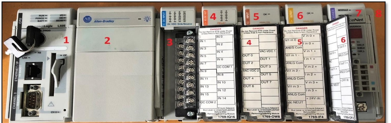
Fig: Compact Logix "1769-L32E" DC I/O + AC I/O + Device Net
