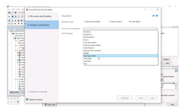
Step 19: Provide an initial display from the application.
