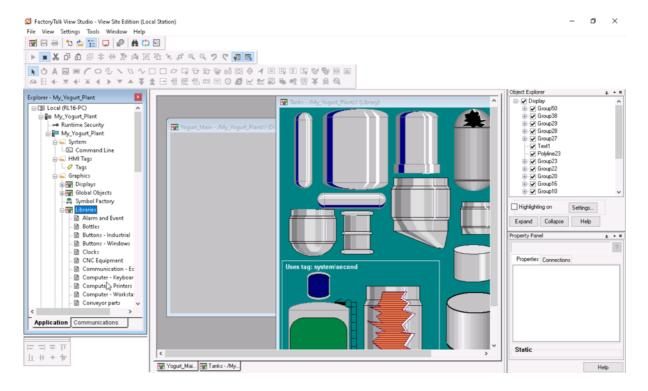
Step 8: By right-clicking on an object, you can copy it and then paste it in the display
