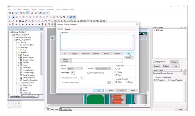
Step 12: You can navigate and search for available tags. For simplicity you can select the "Second" tag as a system variable that could be used to simulate changing variables.
