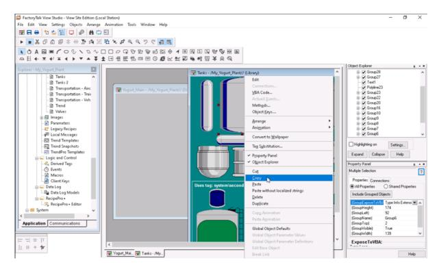
Step 9: Paste an object on the display
