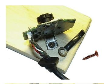
Discard the rubber grommet cutting with the clippers. (Be careful not to damage the cable insulation)
