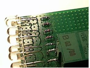
The height of the LEDs from the table top must be more or less the same as the entry slit of the spectrometer. The inlet slit must be covered with diffusion filter otherwise the location of the LEDs become too critical.
