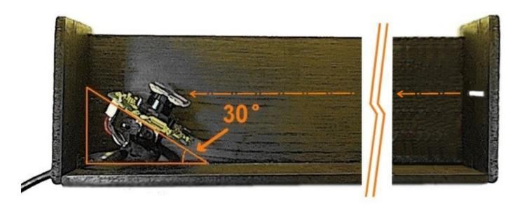
The inlet slot of the light must be horizontal and more or less at the height of the tip of the lens.
