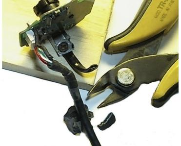
Use the lug to secure the cable, as shown at right.
