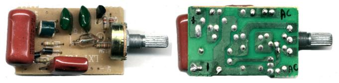
In the original circuit the potentiometer regulated the frequency of the pulses, but it was not possible to exceed 8 or 10 Hz. (Wiring diagrams are on the next page)
