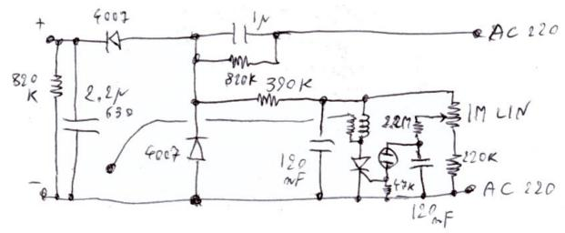
**Original:** The maximum frequency was 8 Hz and the energy of the lightning was unstable, because the flashes were not synchronized with the 50Hz mains.
