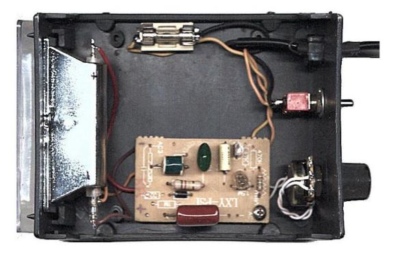
It is a good idea to fix the circuit with a screw (it was originally attached to the potentiometer and rather unstable). And also add a power switch and a fuse holder. A 1 Amp fuse is fine but you could try to get down to 200 mA.
