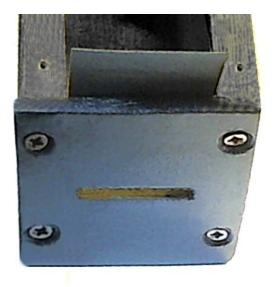
When screwing the lid leave the right space for the diaphragm.
