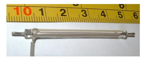
Note the gray paint that covers the conductive wire of ignition and extends along the lamp. Be careful not to overexert this thread, because the paint may crack. In this case begin to twinkle in the breaks and flashes become unstable.
