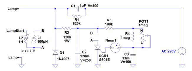
**Modified:** The flashes are synchronous with the 50Hz and the knob adjusts the intensity of the produced light.
