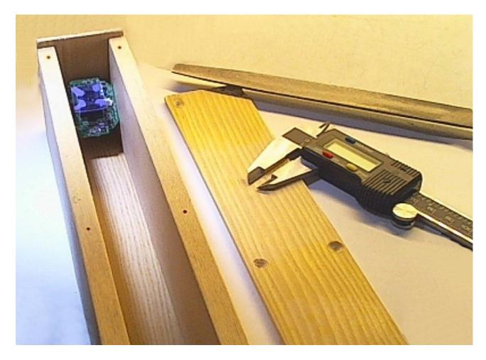
With wood and small screws you can build lightweight containers, easy to open on each side and easy to modify for the tests.
