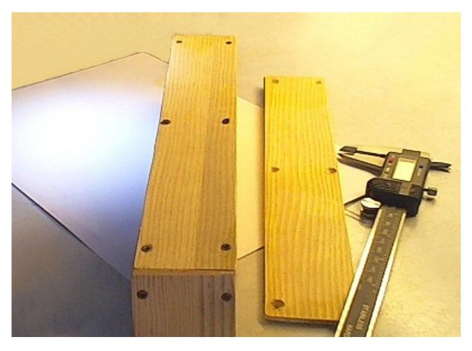
All holes must be made on the 4mm pieces. On the two long pieces you make six holes, three on each side. On the two terminal will make four holes. The holes should be done with a 2.5 mm tip and all must be 5 mm from the edge. Finally, the holes should be flared with a drill bit large (about 6 mm).
