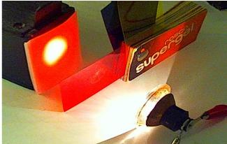
With an incandescent bulb, ranging from 500 nm to infrared energy but below 450 nm is very little and there are significant differences in intensity between different areas of the spectrum.
