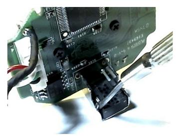
If the button terminals were attached to the PCB, cut at the base, with small scissors or clippers.
