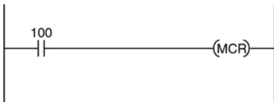
Figure 1.8 Master Control Relay
