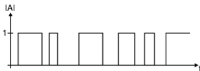
Figure 3.35 A Pulse Density Modulated Waveform
