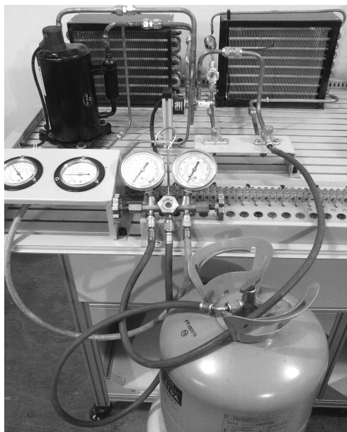
Figure 3-72 Connect the nut to the small refrigerant cylinder
